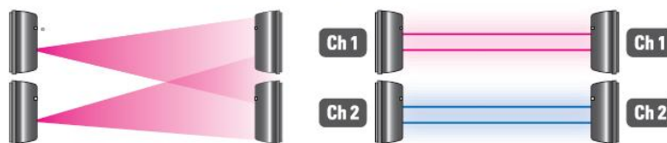
Conventional Beam Sensor (Confusion occurs among beams)
